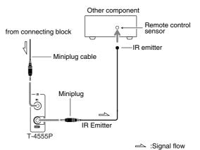
Only remote controller signals received by the T-4555P's IR IN are fed through to the IR OUT. Signals picked up by the T-4555P's remote control sensor are not output.
